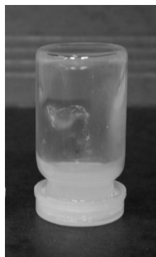
Figure 13. Picture of the final latex obtained from experiment C8 ( t = 3 h, x = 75\% , 28.9 wt % monomer content, [P(MAA_{32-co}-S_4)-SG1]_0 = 1.08 \times 10^{-2} \text{ mol L}^{-1}_{\text{water}} ) (see Tables 1 and 2).
